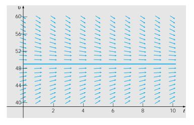
**FIGURE 1.1.3** Direction field and equilibrium solution for Eq. (5).
