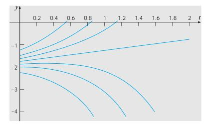
**FIGURE 2.1.3** Integral curves of y' - 2y = 4 - t.
