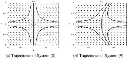
Figure 7.4: Saddle separatrices lie along the axes in (a); two of the separatrices are bent to the right by a nonlinearity in (b).
