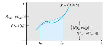
**FIGURE 8.2.1** Derivation of the improved Euler method.
