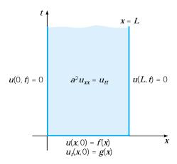
**FIGURE 10.7.2** Boundary value problem for the wave equation.
