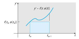
FIGURE 8.1.1 Integral derivation of the Euler method.
