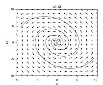
Figure 6.4: Phase portrait of a spiral source:  $x'_1 = x_2$ ,  $x'_2 = x_1 + 0.4x_2$ .
