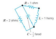
**FIGURE 7.6.3** The circuit in Example 2.
