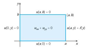
**FIGURE 10.8.1** Dirichlet problem for a rectangle.
