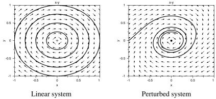
Figure 7.3: Nonlinear terms convert a linear center to a nonlinear sink.
