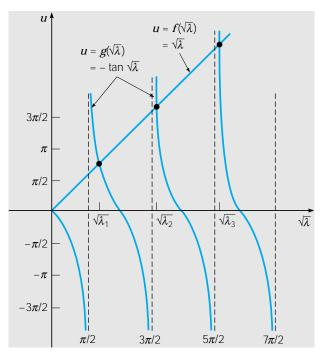
**FIGURE 11.1.1** Graphical solution of  $\sqrt{\lambda} = -\tan \sqrt{\lambda}$ .
