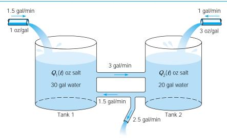
**FIGURE 7.1.6** Two interconnected tanks (Problem 21).
