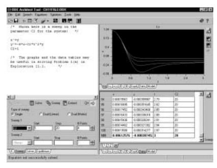
Figure 11.3: Here are some typical graphs for the solution of  $x'' + C_2t^2x' + 9x = 0$  for various values of  $C_2$ . The graphs and the data tables are useful in Problem 1 of Exploration 11.1.
