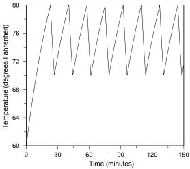
A room heats up in the morning, and the air conditioner in the room starts its on-off cycles.
